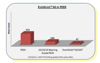
The result of the wear test for PPS demonstrates that the EverGlide® SG offers almost 7x the wear performance of PPS itself and more than 2x the wear properties of the incumbent technology. When we evaluated the EverGlide® SG in PEEK, the technology improved the wear properties 10x while offering almost 3x the performance of the incumbent technology.
