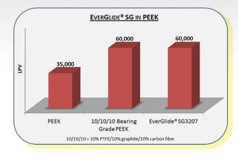
As the charts demonstrate the EverGlide® SG technology not only out performs the incumbent wear technology, but it offers synergies with other technologies to allow for compounds with far superior wear properties.
